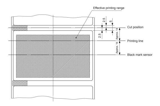
• Min. Label Pitch / Cut Position / Printing Line / Black Mark Sensor's Positional Relationship
